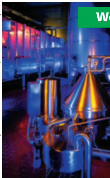
Westfalia Separator Model MSE 500 with HyVOL Protein-Plus System
